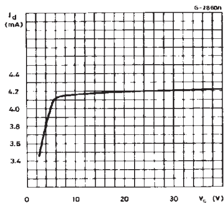
Figure 4. Quiescent Current vs. Supply Voltage.
